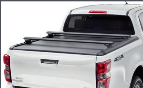
Cross Bars (Black) for RollerTonneau Cover (Compatible with Manual & Electric RollerTonneau Covers. Also available for X-TERRAIN)
