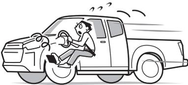
If the brakes unexpectedly stop working, reduce speed by quickly shifting gears down incrementally to 1st gear. Gradually pull the parking brake lever while firmly holding on to the steering wheel and stop the vehicle on the side of the road. After stopping the vehicle, immediately contact the nearest Isuzu Dealer.
