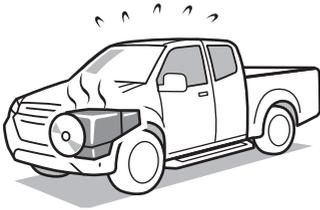
4. Check the engine coolant level in the reserve tank and radiator after the engine has sufficiently cooled. If the level is insufficient, add engine coolant. Also, check to see if the fan belt is loose or has been damaged.
