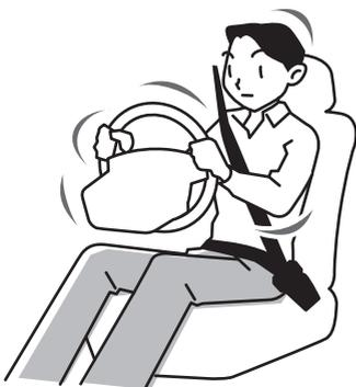
Grasp the steering wheel with both hands, and move it in the axial direction and also up and down, and left and right to see if there is any looseness.
